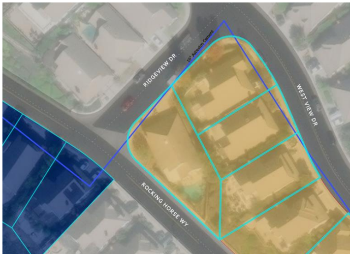
Figure 2. Poor main alignment.
